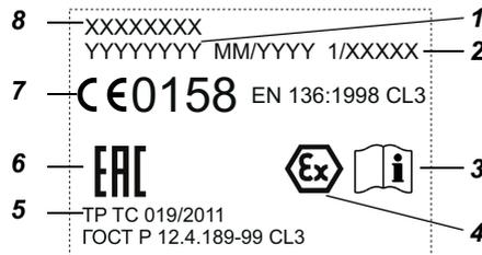
Fig. 3 Marking of mask body
